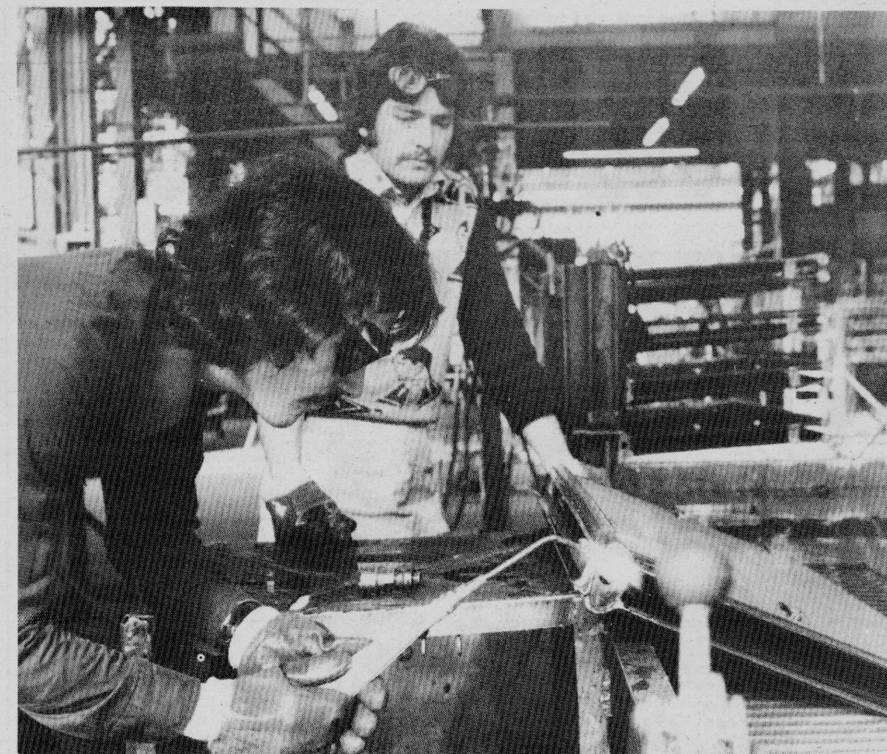
THE WORK of these two men shows the different viewpoints in the co-op. They are radiator testers. They dip radiators into the tank of water, pump air into them and watch for bubbles. If there are any bubbles they weld up the holes in the radiators.
